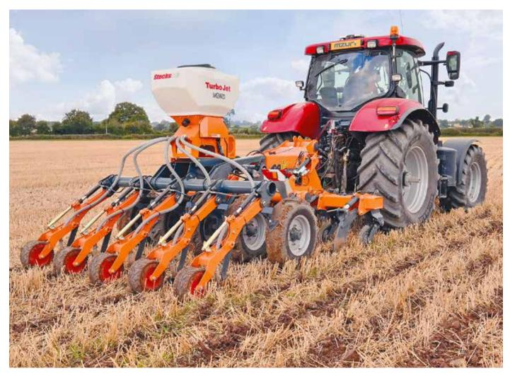
The REHAB subsoiler is available with an option of a seeder unit – ideal for drilling oil seed rape and cover crops. The individual coulters give an accurate sowing depth into a friable seedbed; this provides the ideal soil environment for each seed, ensuring rapid and even germination.
